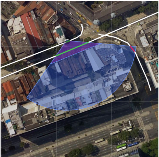
ROTS is calculated as the traffic inside the Visibility cone (blue area) and Obstacles area (purple area)
